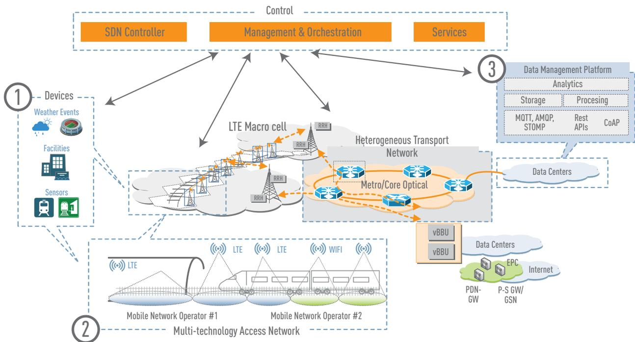
The objective of the Integrated Communication Platform is to define, appropriately model and implement a dynamic network communication platform interconnecting a variety of on-board and trackside sensing/monitoring devices to the railway operations and support centre as shown in the figure above. More specifically the figure shows a use case where data is collected from various devices (1), transmitted over a 5G network (2) to the cloud based data management platform (3)
