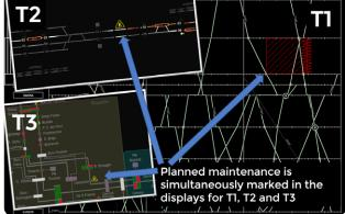
The operators shifts trains between tracks to accomodate for maintenance works
