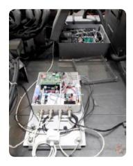
**FIGURE 5** — Installation of the acquisition box Aloha V1 on tram's roof
